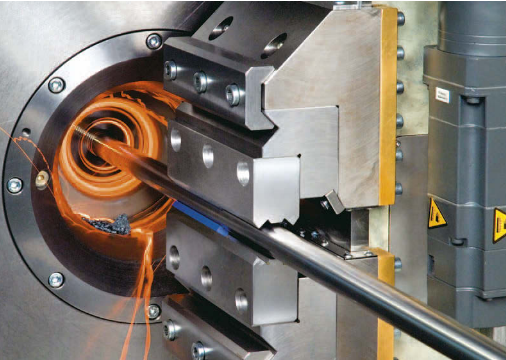
Thread whirling machine with torque motor (type RI)
