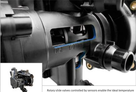
Rotary slide valves controlled by sensors enable the ideal temperature window for the engine and transmission to be reached quickly.
