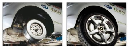
In the *Schaeffler Hybrid*, Schaeffler presents the innovative in-hub motor *eWheel Drive*. It also allows the development of completely new vehicle architectures.
