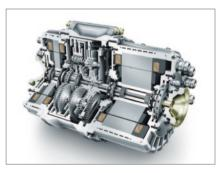
The heart of the ACTIVeDRIVE is the eDifferential. This is an active electric differential. It provides drive power for the vehicle as well as allowing power distribution between the wheels on an axle.
